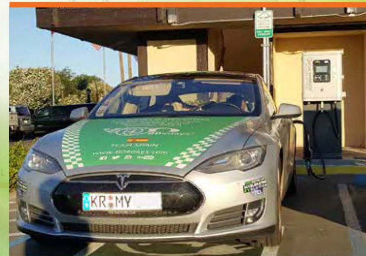
A Tesla Model S can be charged at the EV Express using a CHAdeMO adapter
